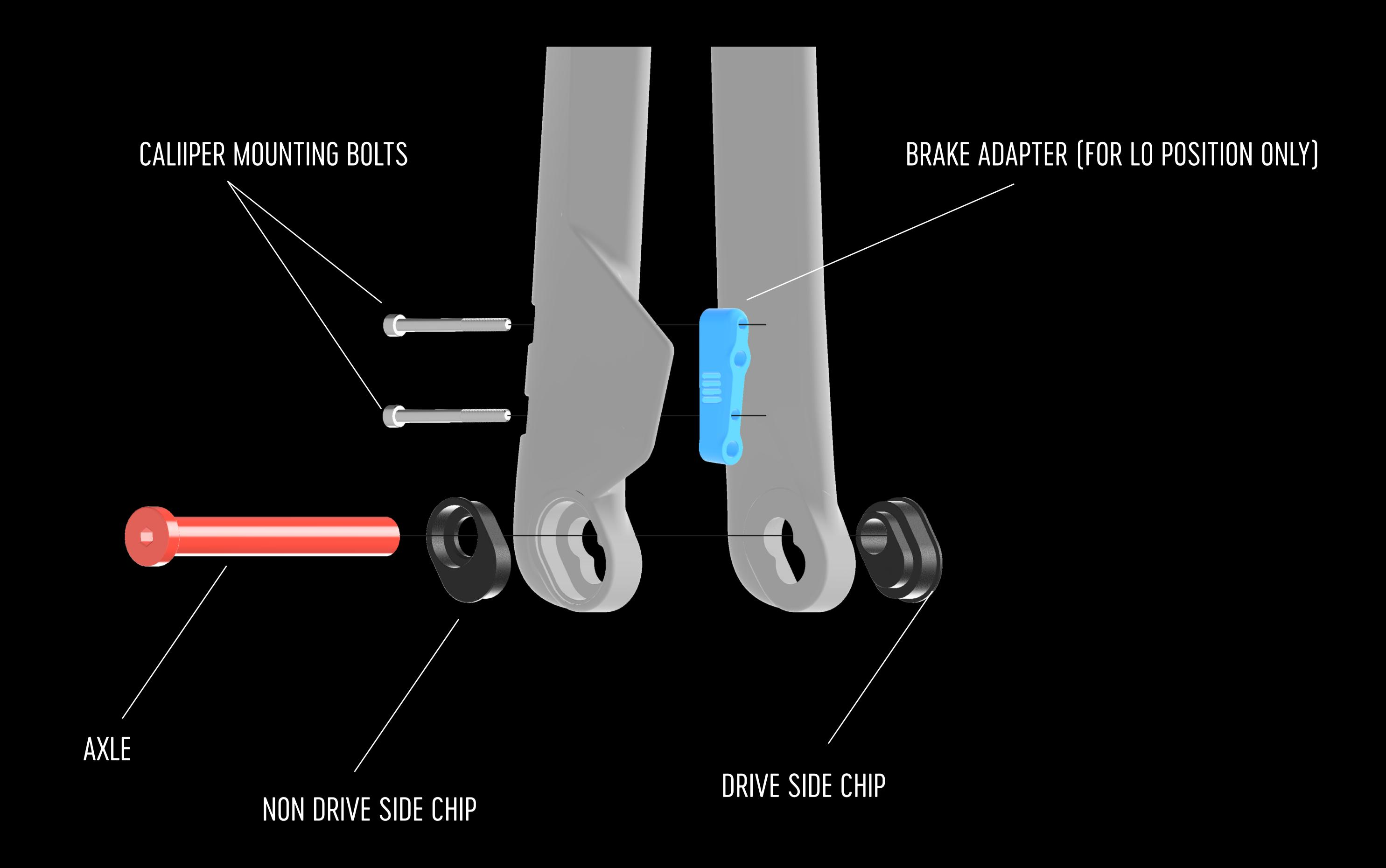
HVRT TWIN TIP as fitted to Rondo HVRT and MUTT bikes MY2020 and newer. Features:
