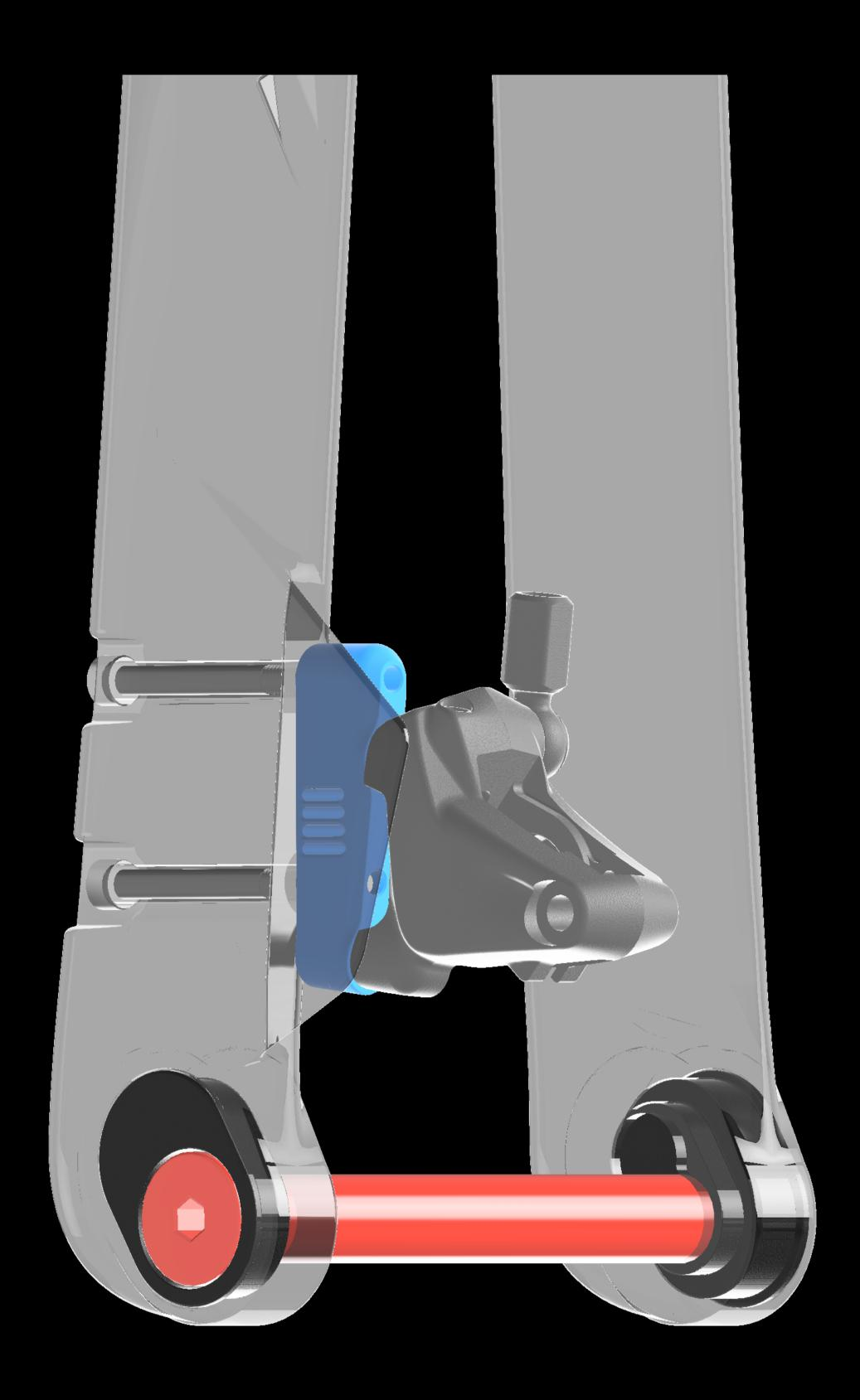
**LO** position provides 380 mm fork length and 40mm offset Your bike will come from the factory assembled in this position by default.
